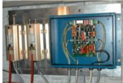
Actuators and control unit on board the test ship "Dintelwerken"
